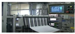
The glass medium is inserted into a computerized Pleating machine where it is precisely folded
