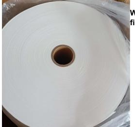
We start with a roll of the specially manufactured glass fiber filter material you see on the left
