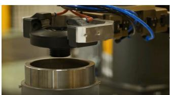
The 2 parts of the black filter cartridge are press fitted together and sealed shut
